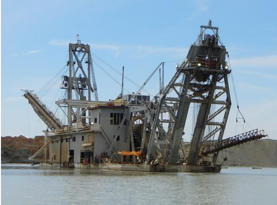
Figure 108. Large scale Gold dredger
