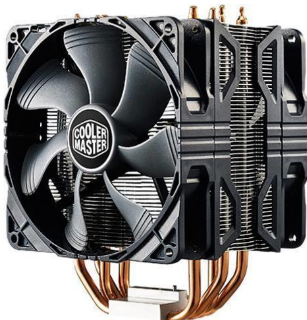
Figure 123. A heat sink in computers and other electronic systems
