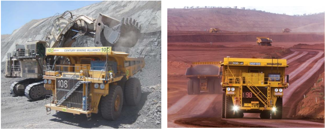
Figure 127. Trucks loading and transporting iron ore to iron processing plants.
