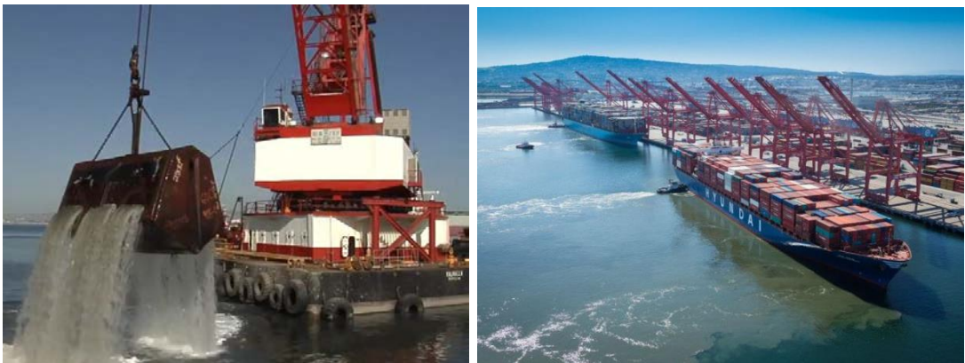
Figure 54. Right, a dredger removing soil and rock deposits around Long Beach Harbour, California USA. LEFT, ships on the Port of Long Beach.
