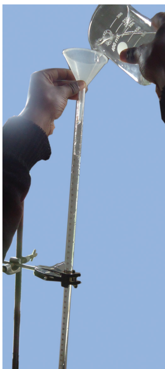
Fig 1.4: Correct filling of burette
