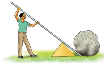
Examples of first-class levers in use
